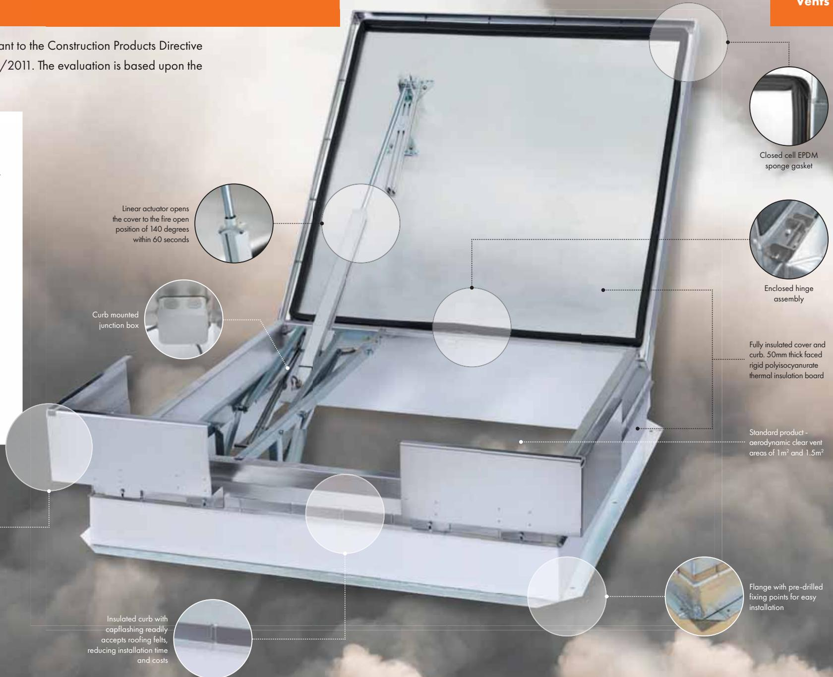
Linear actuator opens the cover to the fire open position of 140 degrees within 60 seconds
