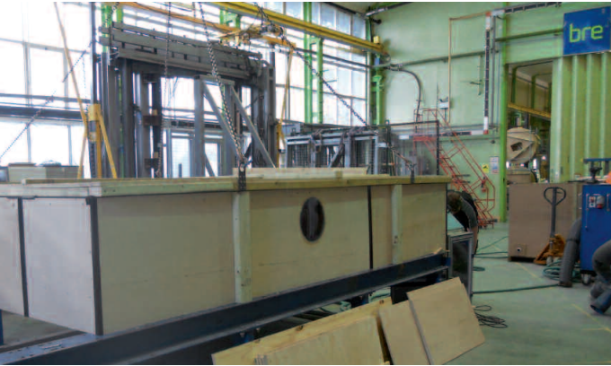
Test apparatus built around specimen and pressurised
