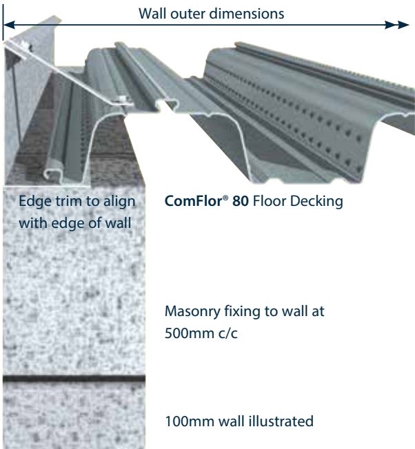
Typical wall side detail
