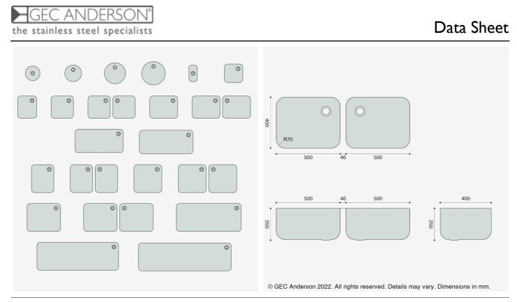
DG54 double bowls: 500x400x250mm. Complete with Ø38mm waste and overflow fittings.
