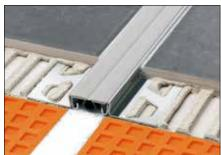
Schlüter®-DILEX-KSBT is a structural movement profile with edge protection. The profile's anchoring legs, made of aluminium, or stainless steel, are connected to a 20 mm or 30 mm wide movement zone made of soft synthetic rubber (see product data sheet 4.19).
