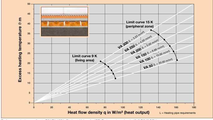
Performance test according to DIN EN 1264, Stuttgart University, IGE, Test report number L.1210.P.943.SCH
