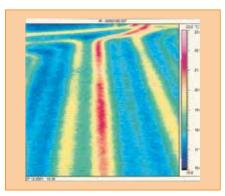
3 The picture was taken after 30 minutes of operation. Average surface temperature above the heating pipe: 21 °C. The heat distribution within the uncoupling mat Schlüter®-DITRA 25 shows a clear temperature increase between the heating pipes.
