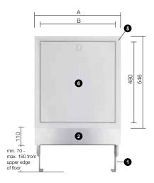
Schlüter®-BEKOTEC-THERM-VSE is a distributor cabinet for in wall installation to fit a Schlüter heating circuit distributor and the associated control components. The distributor cabinet is made of galvanised steel with two stabilizing double edges and pre cut openings in the sidewalls for routing connector cables. The set includes:
