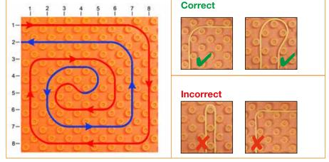
In spiral installations, the heating pipe is installed at double the installation spacing to the reversal loop. After reversal, the return leg is installed in the remaining spaces, which results in the desired pipe spacing.
