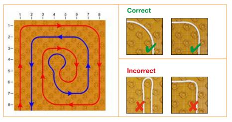
The system heating pipes (Ø 10 mm) are installed at double the installation spacing to the reversal loop. After the reversal point, the return line (blue) is inserted into the centre of the remaining space. **Important:** Form the heating pipes as shown in the drawing!
