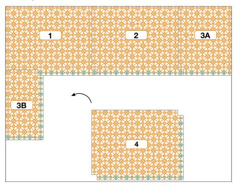
The installation direction is indicated by the tapered connection studs, which are shown in green colour in the drawing. Cut segments that are longer than 30 cm can fit into the next row.
