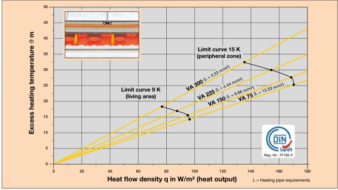
Performance test according to DIN EN 1264, Stuttgart University, IGE, Test report number L.1210.P.957.SCH
