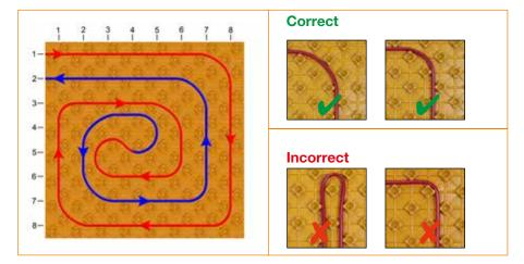
The system heating pipes (Ø 12 mm) are installed at double the installation spacing to the reversal loop. After the reversal point, the return line (blue) is inserted into the centre of the remaining space. **Important:** Form the heating pipes as shown in the drawing!
