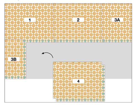
The installation direction is indicated by the tapered connection studs, which are shown in green colour in the drawing. Cut segments that are longer than  $\geq$  30 cm can fit into the next row
