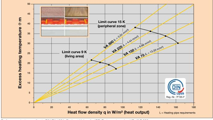
Performance test according to DIN EN 1264, Stuttgart University, IGE, Test report number HB 12 P 380
