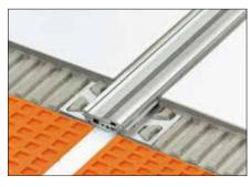
Schlüter®-DILEX-BT is a structural expansion joint made of aluminium, with opposing support profiles that connect to a sliding telescopic centre section. This allows for the absorption of three-dimensional movement (see product data sheet 4.20).
