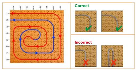
The system heating pipes (Ø 14 mm) are installed at double the installation spacing to the reversal loop. After the reversal point, the return line (blue) is inserted into the centre of the remaining space. Important: Form the heating pipes as shown in the drawing!
