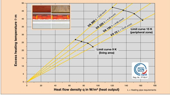
Performance test according to DIN EN 1264, Stuttgart University, IGE, Test report number HB 12 P 380
