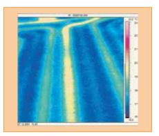
2 The picture was taken after 20 minutes of operation. Average surface temperature above the heating pipe: 19.5 °C. The heat distribution within the uncoupling mat Schlüter®-DITRA 25 shows first temperature increases between the heating pipes.
