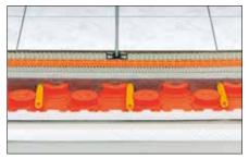
Schlüter®-BEKOTEC-EN System heating pipe  $\emptyset = 16 \text{ mm}$
