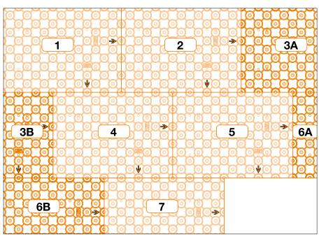
Installation process (with optimal use of material)
