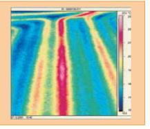
4 The picture was taken after 40 minutes of operation. Average surface temperature above the heating pipe: 22.5 °C. The heat distribution within the uncoupling mat Schlüter®-DITRA 25 provides an even surface temperature and low heat fluctuations.
