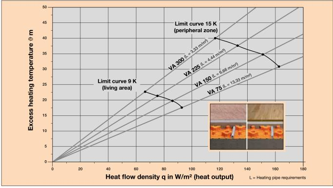
Performance test according to DIN EN 1264, Stuttgart University, IGE, Test report number HB 12 P 379
