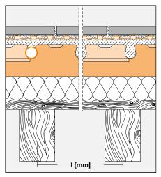
The studded screed panels EN 12 FK and EN 18 FTS are installed exclusively on fully load bearing substrates - not over insulation layers.
