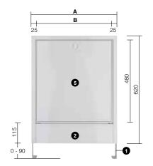
Schlüter®-BEKOTEC-THERM-VSV is a distributor cabinet for wall installation to fit a Schlüter heating circuit distributor and the associated control components. The distributor cabinet is made of galvanised steel, and is powder coated on the inside and outside.
