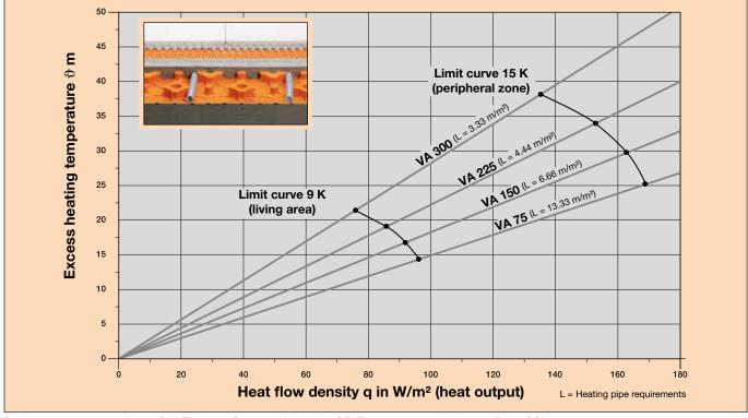
Performance test according to DIN EN 1264, Stuttgart University, IGE, Test report number L.1210.P.950.SCH
