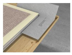
At the beginning of the installation, mark the shower tray to indicate the height difference between the subfloor and the tile surface - for this, take the height of the floor tile and the tile adhesive into an account.
