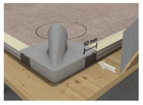
Apply the 520 sealant to the back of the sealing corners, then apply the sealing tape with a 50mm overlap to the corners.
