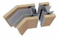
CORNER CONNECTION OF PANELS WITH AN ANGLE OF 135° (GENERALLY 91° TO 179°)
