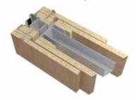
TERMINATION OF A TELESCOPIC PANEL FOR A 120 WALL
