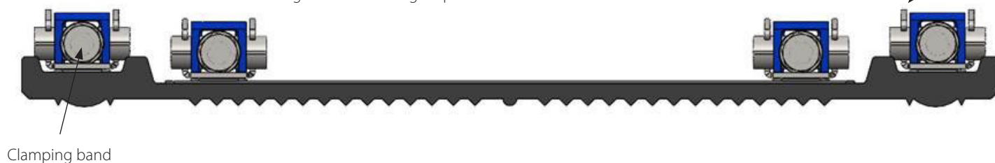
X-Section Through 345mm Sealing Strip
