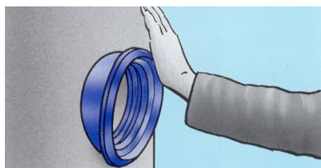
Press the Wall Seal seal into the hole.
