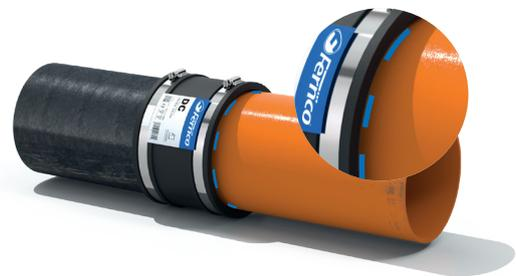
**4.** Position the remaining pipe, ensuring the coupling face and marked line are flush. Tighten this clamp band.
