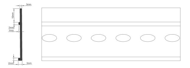
The hidden transition strip has been designed to maintain the overlap detail when replacing flooring without the need to replace the wall system, for installation guidance contact the Altro technical team on 01462 707600.
