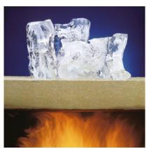
Stone wool does not melt even in a fire. Thus a structure can withstand a fire considerably longer, which can critically improve the chance of rescue and limit damage.
