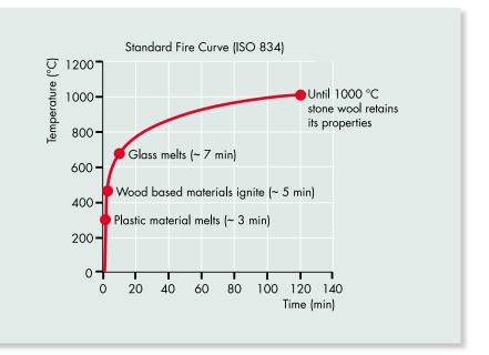
The behavior of certain construction materials in a "standard" fire. A "standard fire" simulates the development of temperature of a fire in normal room space.
