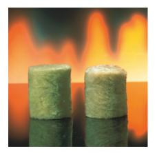
PAROC<sup>®</sup> Stone wool withstands very high temperatures. The image shows a test sample of the PAROC<sup>®</sup> product before and after an EN ISO 1182 non-combustion test where the test sample is burned at a temperature of 750 °C. PAROC<sup>®</sup> UNS are in several of our markets developed into PAROC<sup>®</sup> eXtra<sup>™</sup> with the same fire properties.
