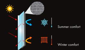
The emissivity of a material is its ability to re-emit the energy received through conduction (heat/cold).
