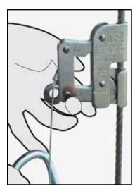
**g.** Ensure the arrow on the shuttle is pointing in an upwards direction and release the latch so the shuttle is held on the cable.
