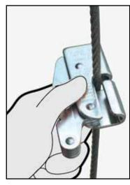
**e.** Holding the shuttle horizontally, position on the cable as shown and rotate the whole shuttle anticlockwise.
