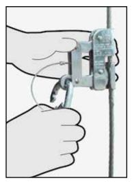
**h.** Take the karabiner and twist the safety clasp in a clockwise direction. Whilst twisting the safety clasp push the karabiner together utilising your thumb as shown.
