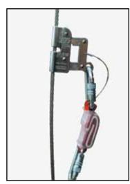
**j.** The shuttle is now ready for the appropriate PPE to be connected to the auto twist locking karabiner as shown above.
