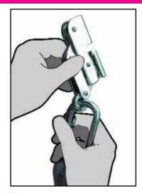
**b.** Whilst twisting the safety clasp push the karabiner together using your thumb as shown.
