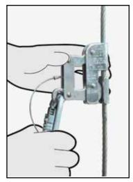
i. Thread the karabiner through the hole in the shuttle and release the karabiner so that it closes and is locked into place.
