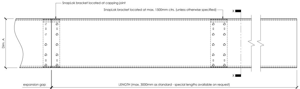
SNAPLOK COMPONENT DETAIL - VIEW ON PLAN
