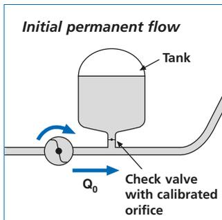
The protective systems that can be installed to limit water hammers to an acceptable level are varied and must be adapted to suit each situation.
