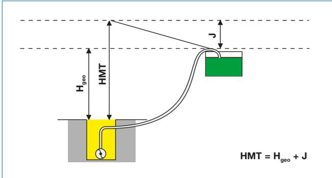
Catchment or storage areas are frequently not high enough to meet the required pressurization conditions. Energy therefore has to be imparted to the liquid to make distribution possible.
