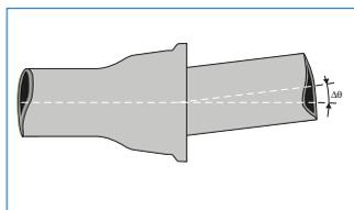
**PAM** SAINT-GOBAIN socket joints allow for angular deflection. In addition to the obvious advantages during laying and to accommodate ground movement, angular deflection allows the incorporation of large radius bends without using fittings, as well as a certain amount of adjustments to the layout.
