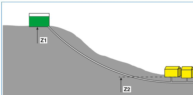
A gravity supply system is the mode of supply which allows water to be driven through a pressure main from a natural or artificial storage area at elevation  $Z_1$ , to all points of supply located at elevations  $Z_2 < Z_1$ , without any energy input.
