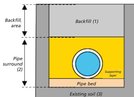
The **pipe surround (2)** protects and/or provides stability for the pipeline.
