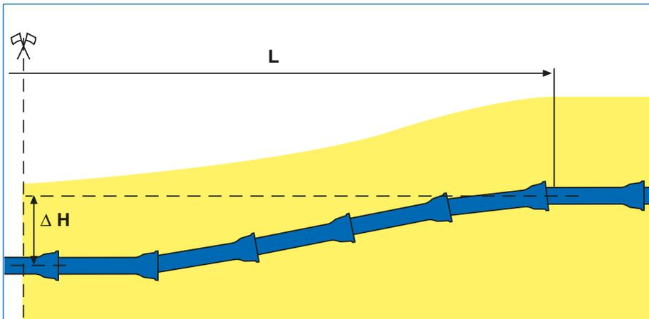
$$\text{Subsidence } \Delta H = 2l \left( \text{tg}\theta + \text{tg}2\theta + \text{tg}3\theta + \dots + \text{tg} \frac{n}{4} \theta \right)$$
