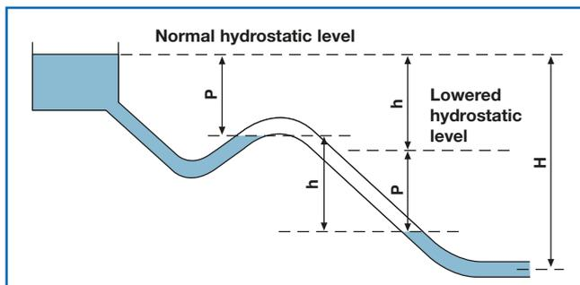
The air pocket transmits static pressure  $P$  from its upstream face to the downstream face and the hydrostatic level drops. Operating pressure  $H$  is reduced by quantity  $h$ , corresponding to the difference in level between the ends of the air pocket and the missing head height.
