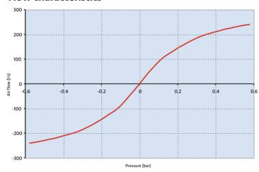
The discharge is as shown both with and without the non-return valve option. The small orifice allows air to escape at a rate of  $5m^3/h$  for  $\Delta P \ge 1bar$ .
