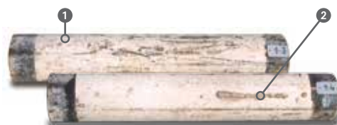
200 g/m 2 zinc + 80 \mu m bituminous paint coating
