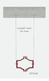
The distance between pipe supports should not exceed 3m, as advised in BS EN 12056-2 Code of Practice for Sanitary Pipework.
