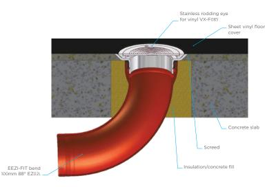
Access to below ground or suspended drainage systems can be designed as simple rodding eye points using Direct Fit gratings. This diagram again shows the flexibility of the PAM ranges of products demonstrating how the grating can connect directly with an EEZI-FIT large radius bend.
