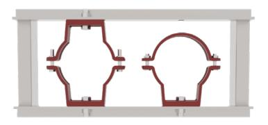
$\label{thm:continuous} \mbox{Typical support arrangement for vertical pipework.}$
