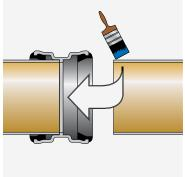
**2.** Place in position and apply force easing coupling into end of pipe until abuts to the central register.
