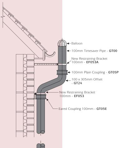
When designing a stack using the new push-fit joint, all fittings require at least one eared socket, to anchor the system to the building. Taking branches as an example, eared joints could be used at the top and bottom of the vertical section to anchor the system, with a plain joint used on the branch arm.
