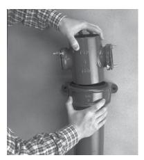
Three joints used on branches can be very close fitting, in some cases they virtually touch. To accommodate this, the plain joint is designed with a flat area which should be lined up with the adjoining socket, to give maximum clearance (see Fig. 39).
