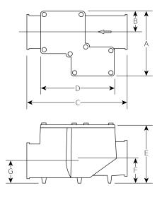
Jones 'Eureka' anti-flooding trunk valves and interceptors for disconnecting chambers and tidal outfalls.
