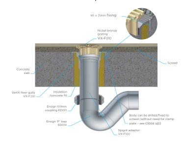
Installations which require a higher level of flow through the grating should use a P trap arrangement which offers less restriction as shown in the diagram. The VortX range of floor gullies, connect directly to the Ensign/Timesaver above and below ground systems using the VX-F500 spigot adaptors.
