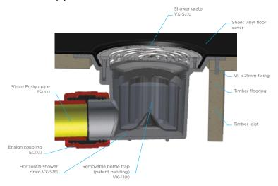
VortX shower drains can be installed in many different applications. Typically the circular gratings VX-S270 are used for vinyl sheet style floor finishes, solid flooring, or timber deck as shown in the diagram. For tiled flooring use the square grates VX-S271. New antiligature shower gratings have now been added to the range – check for availability.
