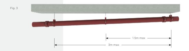
Typical support arrangement for horizontal pipework
