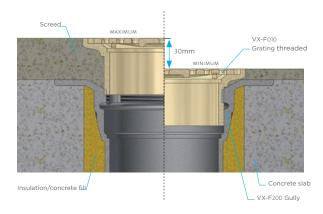
All VortX Nickel bronze and Stainless steel gratings with NPSM threaded spigots allow up to 30mm height adjustment for various depths of floor finish, when screwed directly into the floor gully (as shown). If further height adjustment is needed use in conjunction with VX-F350 NPSM threaded cast iron raising pieces to reach the height required.
