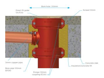
The VortX floor drain range can offer flexible solutions when used in conjunction with the Ensign or Timesaver cast iron drainage system. If there is a need to connect waste pipes from appliances to a back or side inlet – this can be achieved using a direct fit nickel bronze grating connected to an Ensign boss pipe (EF090) using a standard ductile iron coupling EC002.
