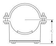
The strap-on boss provides a simple solution for fitting a 50mm copper or waste pipe to an existing 100mm cast iron soil pipe to BS 416 (pipe outside diameter min/max 109/114mm).
