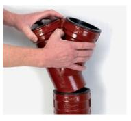
**3.** Apply a small amount of lubricant. Push the second pipe or fitting into the gasket again ensuring that the spigot is abutted against the central register.
