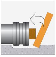
**3.** Apply lubricant to second pipe align with coupling and push pipe until abuts to central register.
