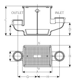
For use inside and outside building. Inside dimensions for TD706:  $455 \times 305 \times 545$ .
