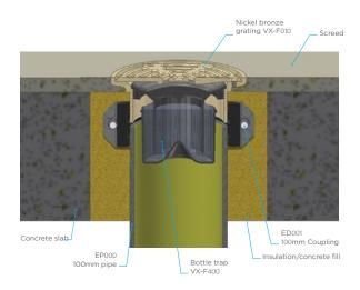
If the grating can be installed in the floor screed without the need for height adjustment then a cost effective option can be to use a Direct Fit grating fitted with a bottle trap. The grating has a spigot of 110mm OD which allows connection to cast iron, HDPE, PVC pipework using a mechanical coupling to suit various ranges ie. EC002 / ED001 / GT01 / TD02.
