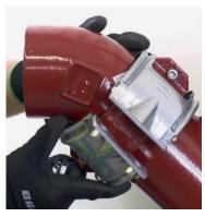
1. Position the two half parts of the PAM Ensign grip collar so to encircle the coupling uniformly. The grip collars must be positioned so that the apertures fit over the fixing bolts of the coupling and the teeth are directly located onto the pipe.
