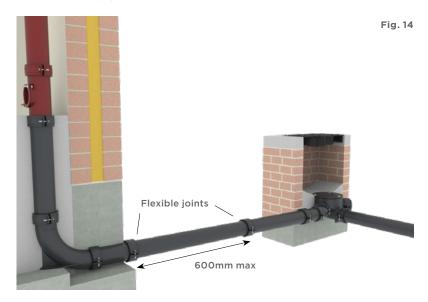
The joint nearest the structure should be as close to it as possible and, in areas where large settlement is expected, more than one 'rocker pipe' may be required (see Fig. 14).
