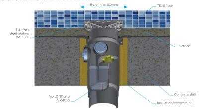
The VortX range includes the innovatively designed S Trap in 100mm diameter which has 3 no. 2" BSP back inlet positions which are supplied plugged off for potential future use.
