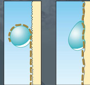
This innovative formula generates a microscopic textured surface with a contact angle of 140°, resulting in a hydrophobic surface. This causes water to bead up into pearls that run across the surface of the facade. As the water runs over the surface of the render, they collect any dirt and contaminants and remove them, cleaning the facade as it rains.
