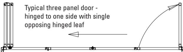
System allows for all door leaves to fold to the internal side only and allows use of fully rebated head and jamb sections, rebated track/threshold profile can be used to provide rebate to all four sides for improved weathering.
