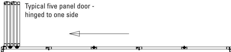
Typical arrangement with sliding folding and single hinged leaf opposite (ok with 3 and 5 panel designs)
