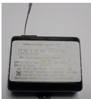
All wireless units must have ONE receiver per operator. The receiver aerial must be fitted outside the operator cover as the signal from the transmitter is blocked by the cover.
