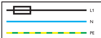
TN-S / TT / TN-C-S Single Phase Supply - Separate Protective Earth & Neutral
