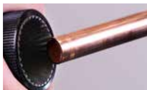
2. Deburr and remove all external sharp edges
