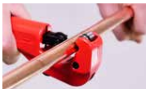
1. Cut the tube to length
