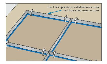
6 Next, the covers should be placed into position, the cover securing bolts should be screwed in (finger tight only) and the 1 mm spacers provided should be inserted between the cover and frame at regular intervals to maintain a nominal 1 mm gap between the covers and outer frame.
