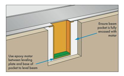
8 The gap between the beam levelling plate and the underside of the beam (standard recessed pockets only) should be filled with an epoxy mortar, maintaining the correct level of the beams.
