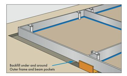
7 Once the above has been completed satisfactorily then backfill under the outer frame and haunch up around the outside with a suitable mortar. Once this has cured then some of the covers can be removed to allow pointing to be carried out under the outer frame from the pit side. Also ensure that the standard type beam pockets are fully encased in mortar.
