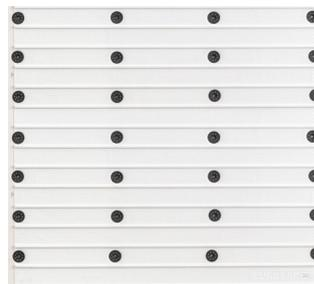
2. Fix panel to substrate using the required number of fasteners; 1 fastener every 2 courses vertically and 4 fasteners across each panel horizontally.
