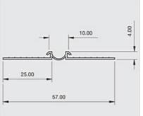
Locally manufactured from recycled plastic, Renderplas PVC movement joint / expansion joint beads are designed for areas of render over 20 square metres and should be specified every 4-6 metres, over structural movement joints and changes of background giving a discreet attractive finish. Also for use as an internal corner with plasterboard
