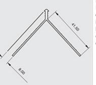
Locally manufactured from recycled plastic, Renderplas PVCu corner beads / angle beads are
