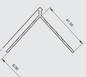
Locally manufactured from recycled plastic, Renderplas PVCu corner beads / angle beads are designed for function and speed on all external and internal rendering and plastering applications. Discreet but strong, all beading gives a perfect finish to through colour render and is equally suitable for sand and cement
