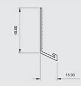
Locally manufactured from recycled plastic, Renderplas PVC bellcast beads / drip beads are designed for function and speed on all external rendering applications. Discreet but strong, all beading gives a perfect finish to through colour render and is equally suitable for sand and cement
