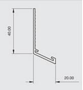
Locally manufactured from recycled plastic, Renderplas PVC bellcast beads / drip beads are designed for function and speed on all external rendering applications. Discreet but strong, all beading gives a perfect finish to through colour render and is equally suitable for sand and cement
