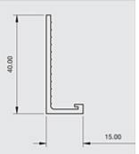
Locally manufactured from recycled plastic, Renderplas PVC stop beads are designed for function and speed on all external and internal rendering and plastering applications. Discreet but strong, all beading gives a perfect finish to through colour render and is equally suitable for sand and cement
