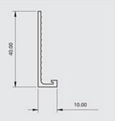
Locally manufactured from recycled plastic, Renderplas PVCu stop beads are designed for function and speed on all external and internal rendering and plastering applications. Discreet but strong, all beading gives a perfect finish to through colour render and is equally suitable for sand and
