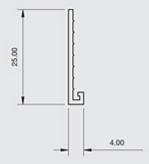
Locally manufactured from recycled plastic, Renderplas PVCu small wing stop beads are designed for economy and speed on external and internal rendering and plastering applications where the substrate is even
