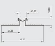
Locally manufactured from recycled plastic, Renderplas PVCu movement joint / expansion joint beads are designed for areas of render over 20 square metres and should be specified every 4-6 metres, over structural movement joints and changes of background. Discreet but strong, all beading gives a perfect finish to through colour render and is equally suitable for sand and cement
