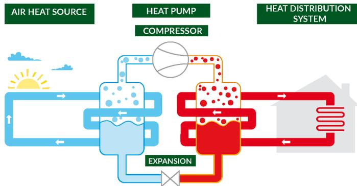
So long as the outside air temperature is above  $-20^{\circ}\text{C}$  heat can be drawn out of the surrounding air to be transferred to a building's heating or hot water circuit. The UK's relatively mild winter temperatures help ensure a properly installed ASHP system can achieve excellent levels of efficiency and performance throughout the year.
