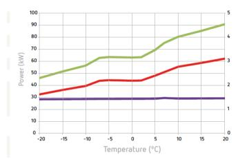
— Power Output (kW) — Power Input (kW) — COP
