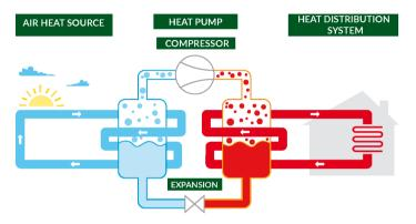
So long as the outside air temperature is above -20°C heat can be drawn out of the surrounding air to be transferred to a building's heating or hot water circuit. The UK's relatively mild winter temperatures help ensure a properly installed ASHP system can achieve excellent levels of efficiency and performance throughout the year.
