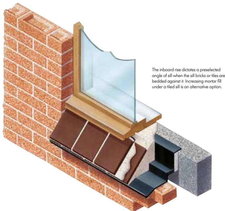
The inboard rise dictates a preselected angle of sill when the sill bricks or tiles are bedded against it. Increasing mortar fill under a tiled sill is an alternative option.
