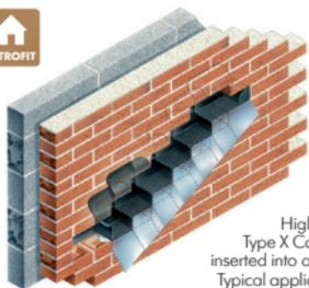
High performance Type X Cavitytrays can be inserted into an existing wall. Typical applications include introduction when a building is added to an existing structure or where the original DPC has failed.
