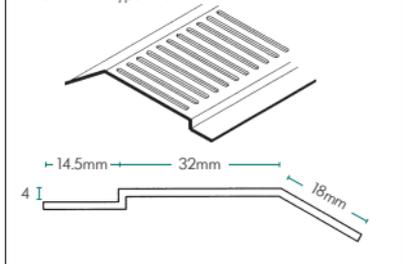
Dimensions of the standard Type SSV, which is for use on roofs of 15 degrees upwards.
