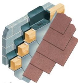
Multicourse cavity trays are available in dimensions to suit all masonry course heights and all thicknesses of external skin. The Multicourse tray style varies pending course height and masonry thickness. The illustration is an example of one such style. Illustrated is left hand long lead tray.
