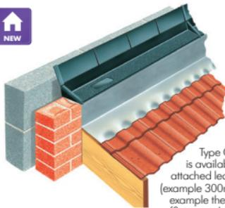
Type G Cavitytray is available with an attached lead flashing (example 300mm.) In this example the flashing is sufficient to dress directly over the abutting roof tiles.
