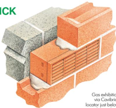
Gas exhibition via Cavibrick locator just below barrier level
