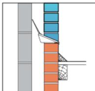
Type E cavitytrays with extended flexible upstands are particularly suitable for non-standard or varying cavities.
