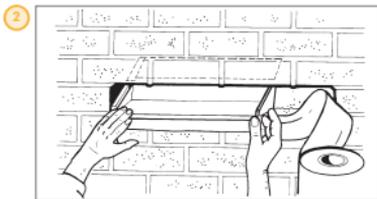
**Step 2** - One cavitytray is inserted together with the flashing intended for dressing over the skirting of the roof finish (flashing approx 50mm into wall).
