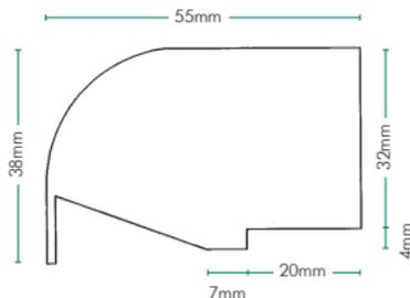
Over Fascia Ventilator OFV25, for roofs requiring the equivalent of a 10mm continuous gap. Suitable for roof pitches of 15 degrees upwards.
