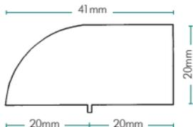
Over Fascia Ventilator OFV10, for roofs requiring the equivalent of a 10mm continuous gap. Suitable for roof pitches of 15 degrees upwards.
