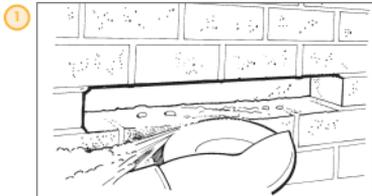
**Step 1** - Three bricks are removed from the wall forming a 675mm opening (an angle grinder/cutter is ideal for cutting out).
