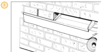
**Step 3** - Two bricks are replaced in the wall into the Cavitytray. They are jointed and securely slate pinned, leaving the wall above safe and firm.
