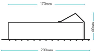
Staggered placement option permits sloping tops and bottoms to interface and eliminate end joining
