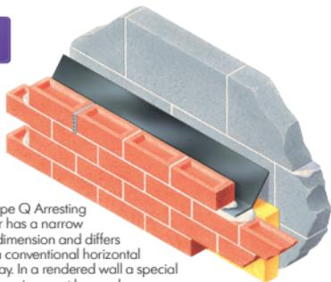
The Type Q Arresting Barrier has a narrow base dimension and differs from a conventional horizontal Cavitytray. In a rendered wall a special wider version must be used.
