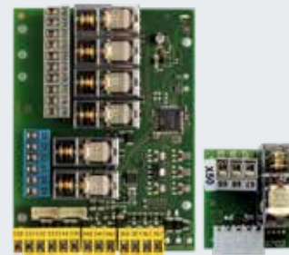
Extension PCB for controls: BK 150 FU E-1 (E FU H) AK 500 FUE-1 (E FU H)
