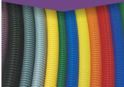
Single wall Polypropylene flexible corrugated 250N conduit can be supplied in standard sizes 20mm 25mm 32mm Coiled in 25m 50m 100m lengths although bespoke lengths can be manufactured to order. Standard colours are
