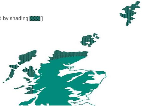
Due to the exceptionally high wind loads which are experienced on the Scottish Islands and exposed Coasts, specific recommendations are required for the use of fibre cement profiled sheets as detailed below. These recommendations should be considered as the minimum requirements for fixing sheets in the shaded area of the map, but where design wind loads exceed 2.5kN/m<sup>2</sup>,
