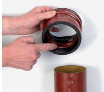
1. Apply a small amount of jointing lubricant on the lip of the rubber gaskets at both ends to ease insertion of pipe/fittings.
