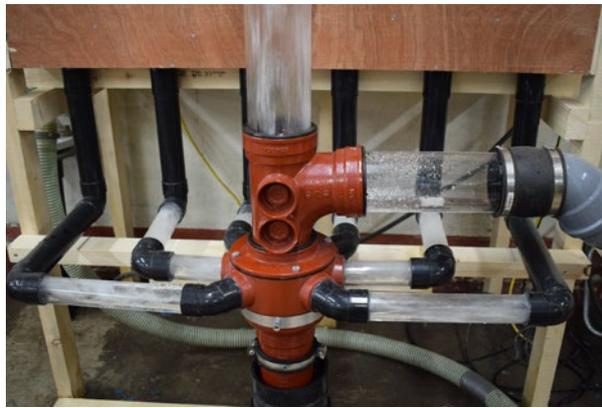
Example how all 6x2" BSP waste inlets being utilised
