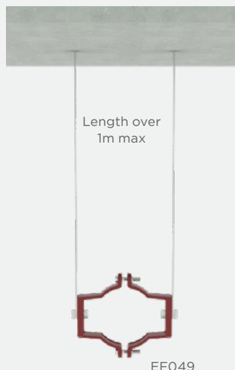
The distance between pipe supports should not exceed 3m, as advised in BS EN 12056-2 Code of Practice for Sanitary Pipework.
