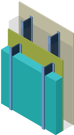
Wall assembly using vertical steel girts
