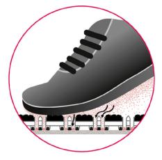
Open structure matting is the most effective design to ensure that dirt and moisture is removed from the top surface, so that it is not carried further into the building by the next wave of traffic.
