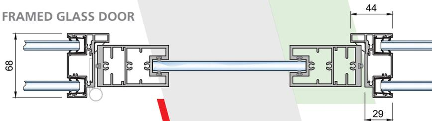
**System 68 Double Glazed Drywall Integration** - QIC System 68 is the only solution for a truly integrated frameless glazed and drywall junction.
