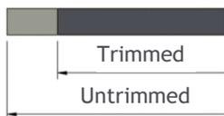
**The panel must not be installed with untrimmed edges.** Approximately 10 mm needs to be trimmed from each of the untrimmed (raw) edges.
