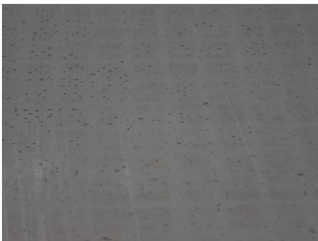
Photo 6 No damage after hard body impact.
