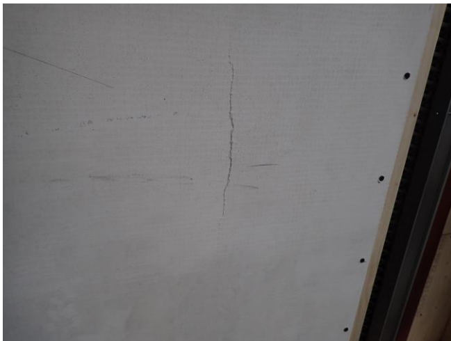
Photo 4 Damage after 300 Nm soft body impact.
