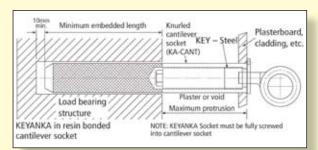
**KEY-CANT** Knurled cantilever socket for use in conjunction with standard **KEY-STEEL KEYANKA** socket in concrete and masonry.
