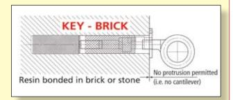
**KEY-BRICK** Standard **KEYANKA** socket with knurled extension suitable for resin bonding into min. 225mm thick solid masonry. NO cantilever permitted.
