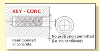
**KEY-CONC** Standard **KEYANKA** socket suitable for resin bonding into minimum 150mm thick concrete ONLY. NO cantilever permitted.
