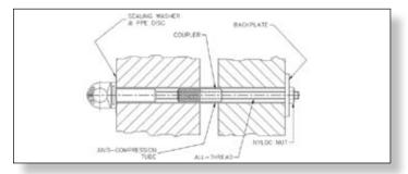
Eyebolt extended with threaded connector and all-thread for use as a through-bolt in solid or cavity wall.
