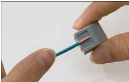
Stripping length Strip conductor by 9 mm
