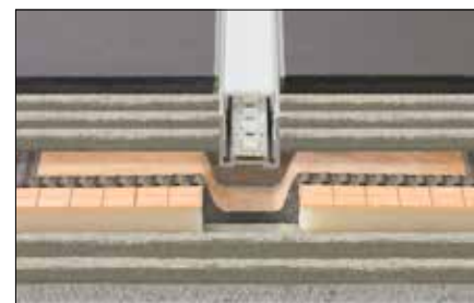
Fig. 2: Schlüter®-LIPROTEC-LL with Schlüter®-KERDI-BOARD-K in a thickness of 10 mm
